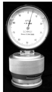
Figure 4. Measuring device for Shore D hardness
