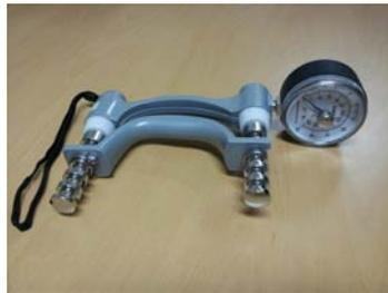
Fig. 2. Tool for measurement of pinch power, Jamar Pinch Gauge(PG60)
