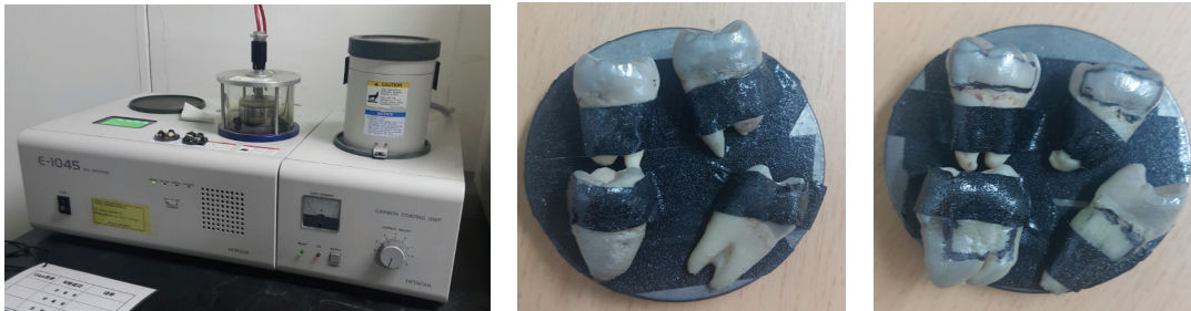
Fig. 2. Test specimen coated with equipment(Hitachi E-1045)
