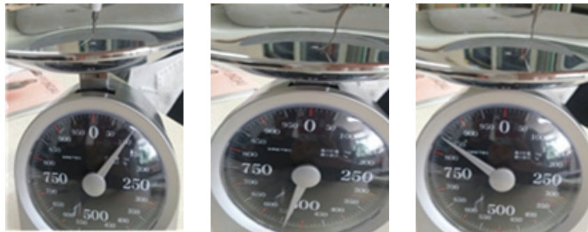
Fig. 3. Lateral pressure measurement using the weighing scales
