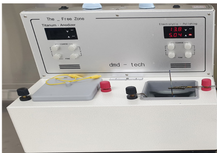
Fig. 3. Electro polisher. Dmd-tech for conducting electro polishing.
